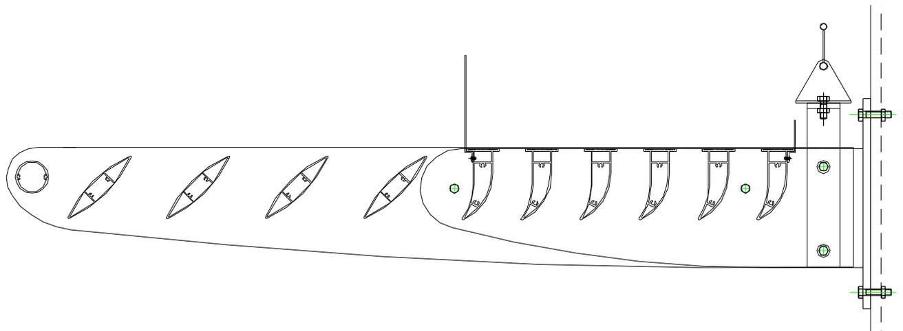
Figure 5 Typical Brise Soleil Incorporating a walkway section
