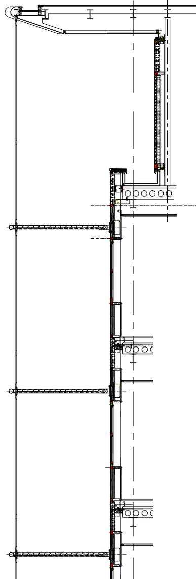
Figure 3 Horizontal Projecting Cable Braced Brise Soleil Installation
