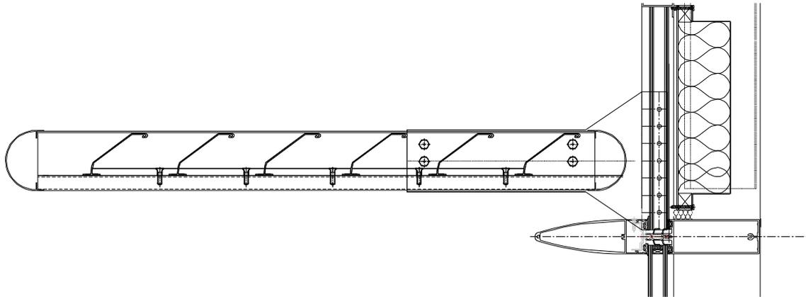
Figure 1 Typical Horizontal Brise Soleil Installation
