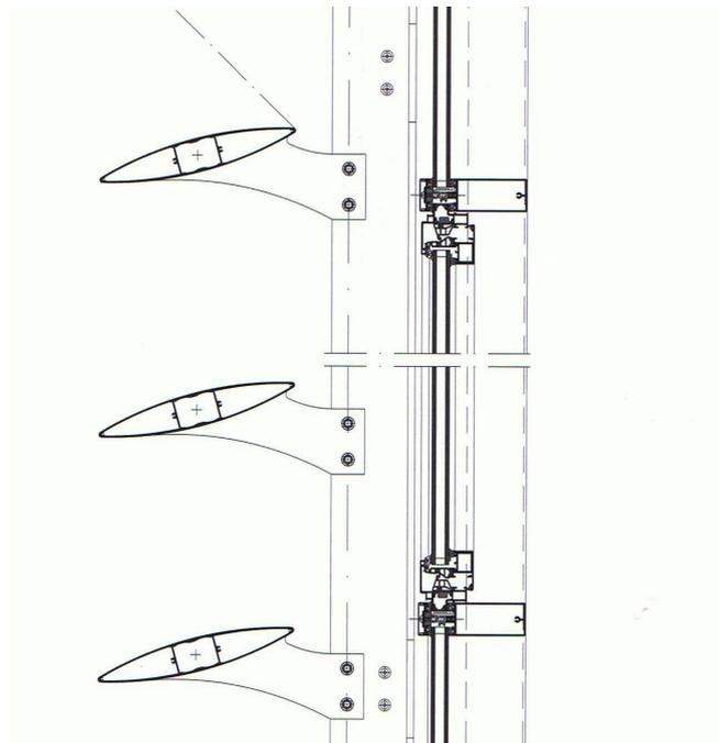
Figure 4 Typical Vertical Brise Soleil Installation
