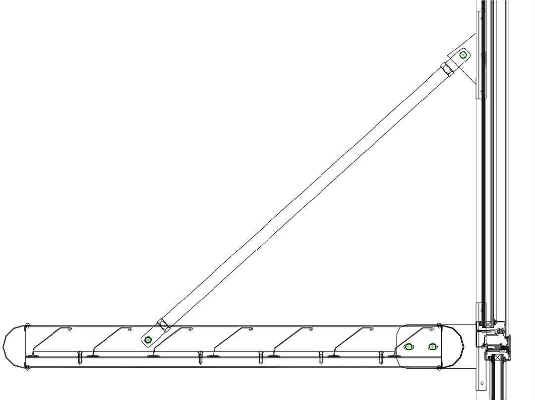
Figure 2 Typical Horizontal Braced Brise Soleil Installation
